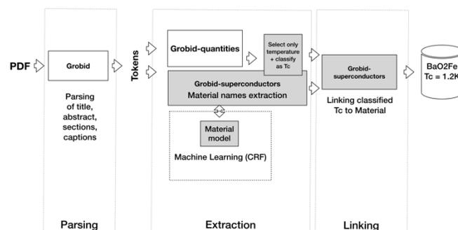
Figure 1: Schema of the system showing the interaction of different component and models when a document is processed.
