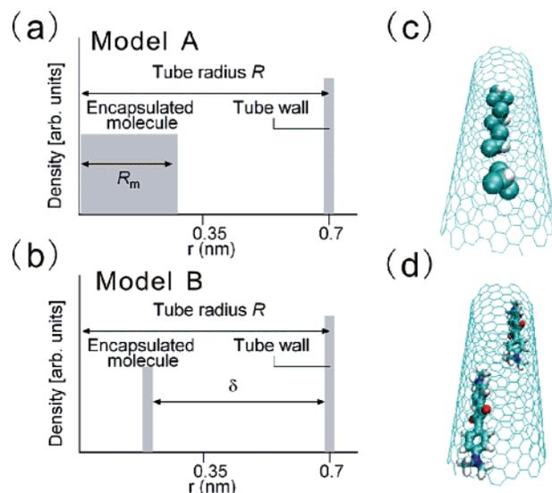
**Figure 3.** Schematic illustrations of (a) model A and (b) model B used for the analysis of the X-ray diffraction profiles of  $\text{CHCl}_3$ @SWCNTs and SQ@SWCNT powders, respectively, and corresponding structural images: (c)  $\text{CHCl}_3$  and (d) SQ dye molecules encapsulated in (12,7) SWCNT.
