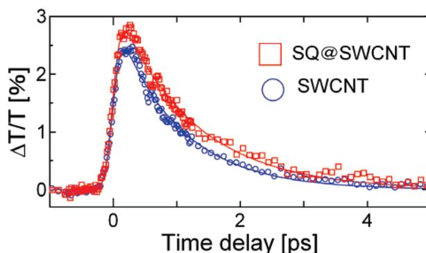
**Figure 9.** Transient transmittance change of the S1 absorption (at 1810 nm) after 708 nm photoexcitation of SWCNT (bottom blue  $\circ$ ) and SQ@SWCNT (top red  $\square$ ) films. Solid red and blue lines are the simulation results for SQ@SWCNT and SWCNT, respectively, using monoexponential functions convoluted with the system response.
