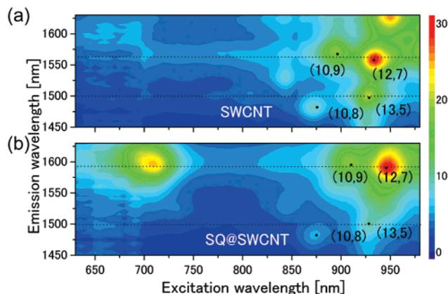
**Figure 6.** 2D maps of the photoluminescence (PL) excitation/emission peak intensities in (a) SWCNT and (b) SQ@SWCNT in SDBS/D<sub>2</sub>O 1% solutions. Dotted lines outline the PL excitation cross-sections shown in Figure 7.
