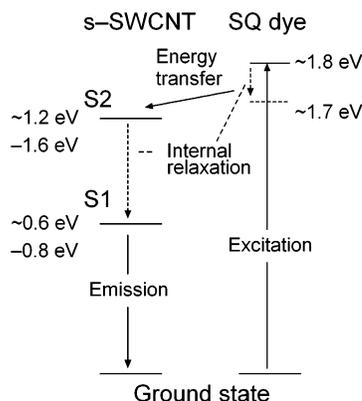
**Figure 8.** Schematic illustration of the energy relaxation pathway after photoexcitation of the SQ dye encapsulated in semiconducting-SWCNTs (s-SWCNT) with  $\sim 1.4$  nm diameter. The energy diagrams are depicted in the exciton picture.
