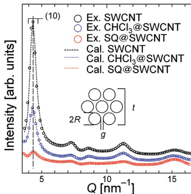
**Figure 2.** X-ray diffraction profiles of SWCNT (black  $\circ$ ), solvent encapsulated SWCNT ( $\text{CHCl}_3$ @SWCNT, blue  $\circ$ ), and SQ dye encapsulated SWCNT (SQ@SWCNT, red  $\circ$ ). Dotted black, blue, and red lines present the corresponding simulated patterns.
