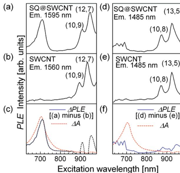
**Figure 7.** Photoluminescence excitation (PLE) spectra of the (10,9), (12,7), (10,8), and (13,5) tubes in SQ@SWCNT (a and d) and SWCNT (b and e) dispersions. (c) and (f) present the difference PLE ( $\Delta$ PLE) spectra (blue line) between the SQ@SWCNT and SWCNT spectra. The line shapes of the SQ absorption band ( $\Delta A$ , dotted red line), which is derived from the difference between the absorption spectra of the SQ@SWCNT and SWCNT, are shown for comparison in (c) and (f).
